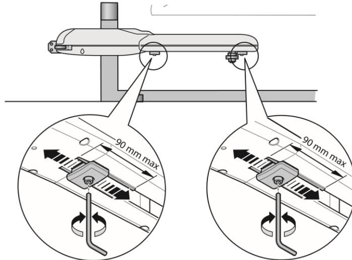
Before continuing to the next step, prepare the ends of travel stoppers on the motor. Each stopper should be positioned to approximately the middle of their range. The maximum range of each stopper is 90mm as indicated in the image here. You will need to use a 5mm Allen® hex key here.
