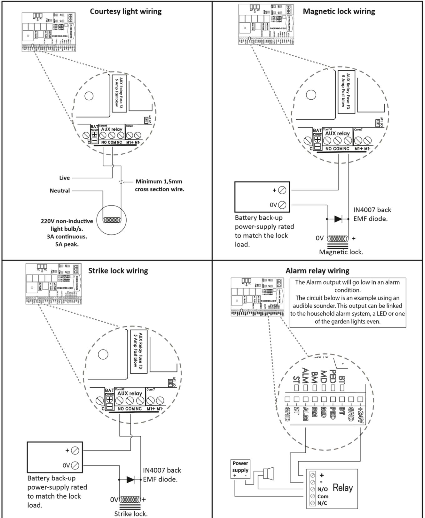
**NB!** Before continuing ensure all wiring and connections are correct and firm. All switching input circuits should be tested using their LED indicators to ensure they are switching correctly and that they are not false triggering.
