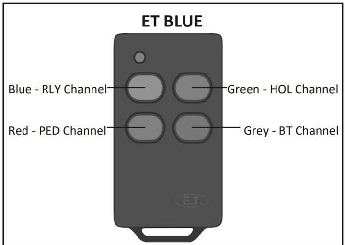
All buttons should be set to either ET BLUE format or ET BLU MIX © format for this to work as shown here.
