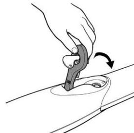
Using the key lock the lever in place.
