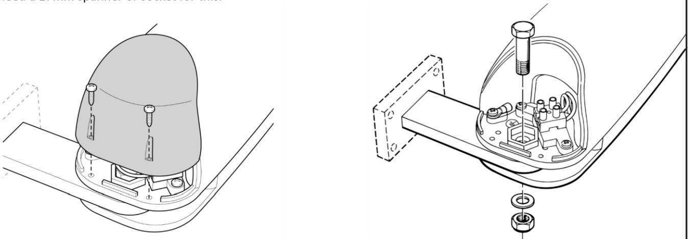
**NB!** Be careful at this step as the motor is only fastened at one end. Provide sufficient temporary support at the gate mount end of the motor to prevent any possible damage to the motor.
