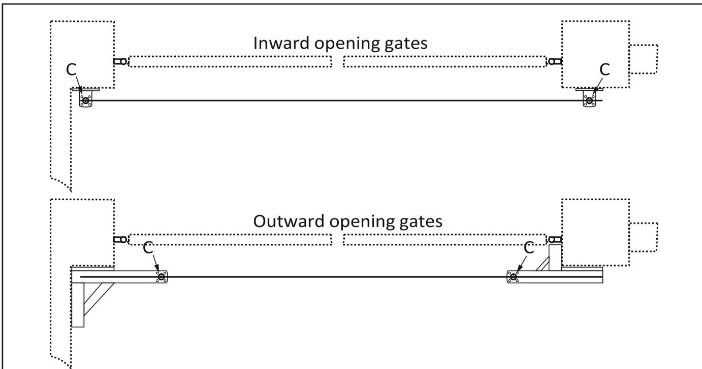
Prepare and install the motor mounting brackets so that the motor head pivot point on the brackets line up with the previously determined positions "C".
