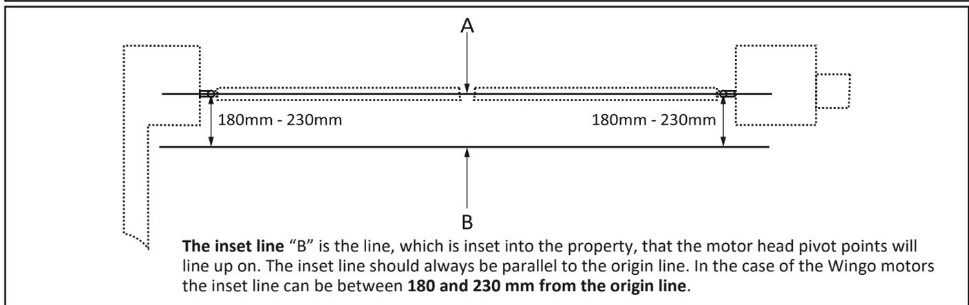
The origin line and inset line are the same in both inward opening gate and outward opening gate applications.
