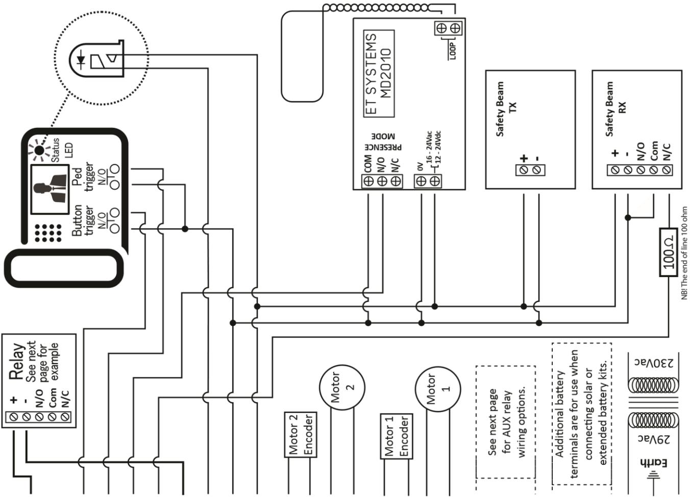
NB! The end of line 100 ohm resistor supplied, must be fitted in the beam receiver as shown here.
