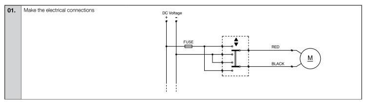
Check that the motor rotates in the desired direction. If not, invert the black wire with the red wire
