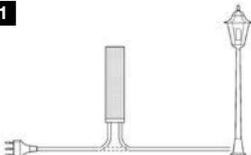
tioned directly in the dedicated compartment. To avoid any risk of water infiltrations, we recommend positioning it with the cables facing down (**Fig. 7**).
