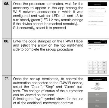
⚠ If the procedure described does not terminate successfully, check that the requirements indicated at the beginning of the manual are satisfied, run the IT4WIFI Reset procedure using the P button (Chapter 8) and then try again.
