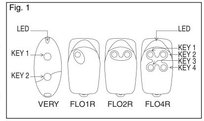
the transmission signal. If the battery is partly flat the LED will give the first pulse and start transmitting only after half a second.
