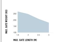
The shape, the height of the gateand the weather conditions can considerably reduce the values shown in the graph to the side.
