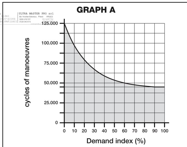
**Example of calculation of durability of a Wingo WG5024 gear motor (refer to Table 2 and Graph A):**
