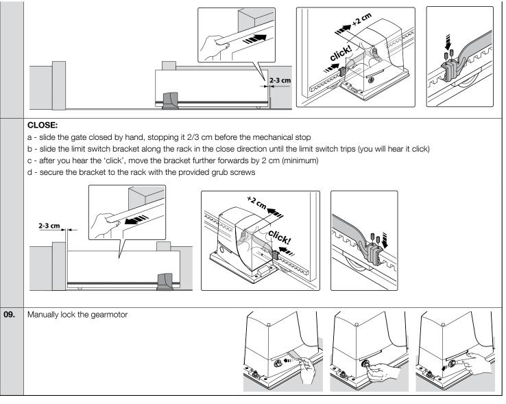
Manually lock the gearmotor.
